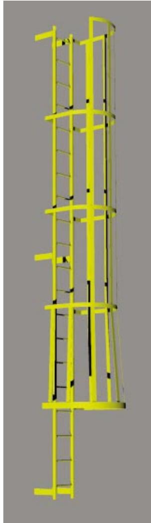
Ladder Length is determined by height of Deck from water surface but no less and 20 Ft. above mean high water.
