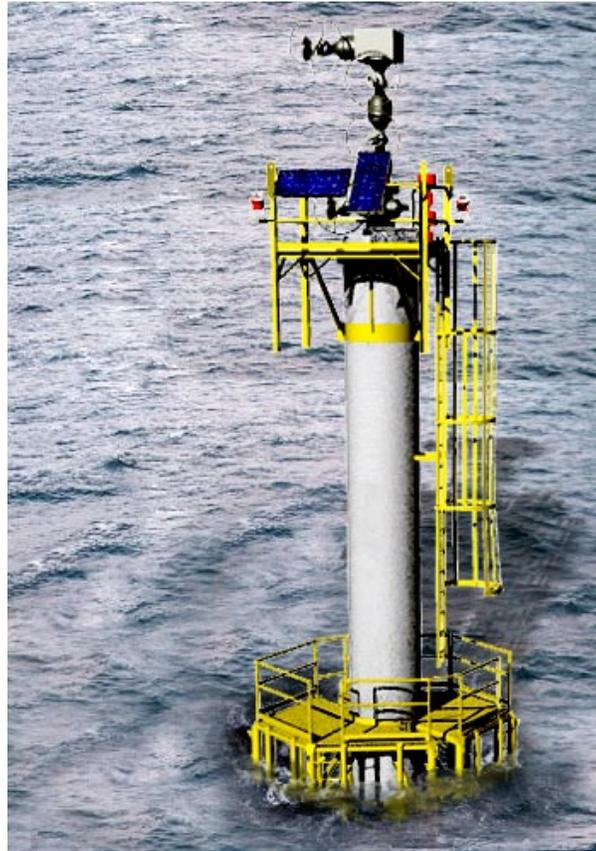
The Essi Corporation (8 Ft. x 6 Ft.) "Clamp-On" Deck With Hand Rails is ideal for remote "satellite well" applications.
