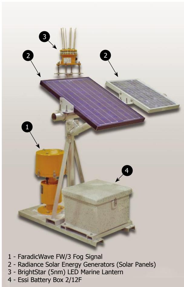
The Essi Corporation Class "B" Single Lift Aluminum Skid is a heavy duty self-contained aids to navigation package powered by batteries and recharged by solar panels.
