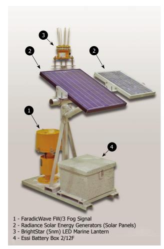
The Essi Corporation Class "B" Single Lift Aluminum Skid is a heavy duty self-contained aids to navigation package powered by batteries and recharged by solar panels.
